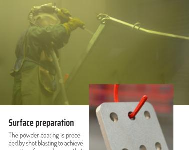
The powder coating is preceded by shot blasting to achieve a matt surface and ensure that the coat of paint can adhere to it perfectly.
