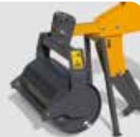
Rear smooth roller with mechanical adjustment
