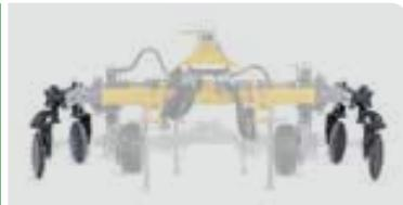
Pair of backfilling discs
