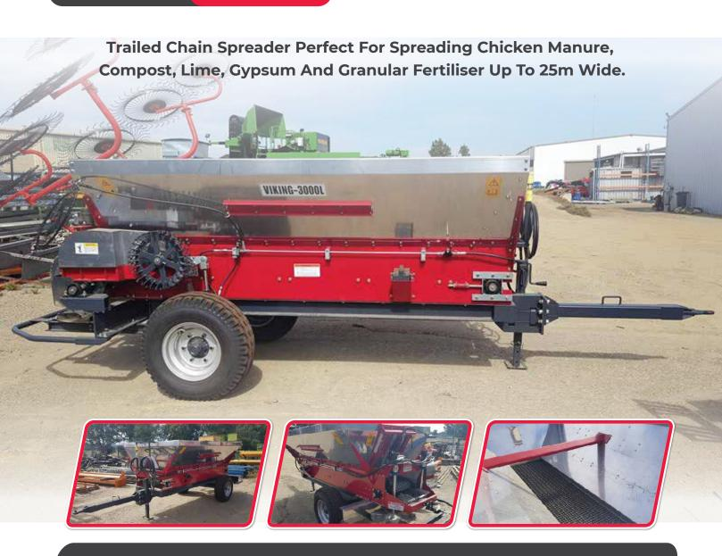
Designed to be low to the ground to fit under vine. Designed to be low to the ground to fit under the vine, ease of loading and a lower center of gravity.
