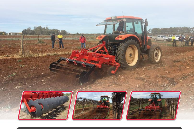
Working speed is generally 10 - 12 Km/h and adjustment of the cage roller can be made with hydraulic cylinder
