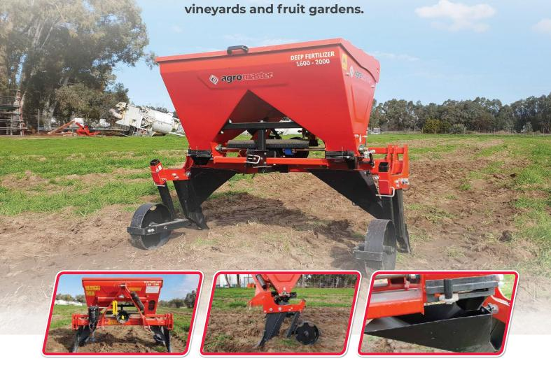
The Agromaster BAF 160 vineyard fertiliser spreader with two fertilising tines that are mounted to the tractor via three point linkage. The space between tines is adjustable and the spreading mechanism can be closed on one side to allow spreading on a single tine.
