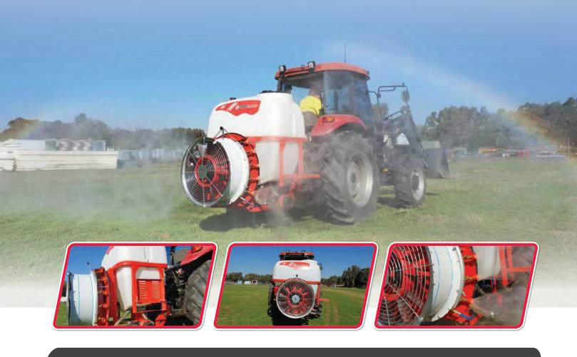
Mounted type 600 L mistblowers are used for multipurpose plant protection. Mistblowers powered by P.T.O. pump delivers the liquid under the pressure to nozzles on the spray fan. Propeller and pump driven by PTO. able to cover trees up to 10-15 meters height. ideal for orchards and vineyards.
