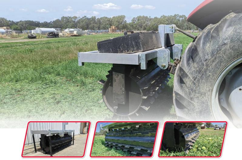
The CropCrimper is designed to terminate cover crops without the need for herbicides. The CropCrimper leaves a mat of mulch that the cash crop is then planted directly through. Crimping leaves a mat (a layer of protective mulch) that aids in retention of moisture in the soil and returns valuable nutrients from the cover crop to the soil.
