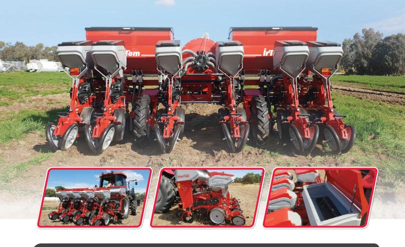
Three point linkage planter ground drive to seeder mechanism with PTO to vacuume system
