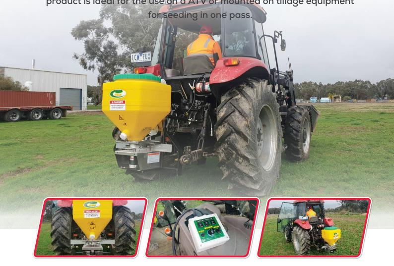
The IE-100 is powered by 12-volt power source making it extremely user friendly and effective way to broadcast seed and bait.
